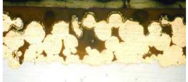
Fig. 12b. Metal-polymer benchmark bearing after corrosion testing
