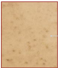
CuSn8 with Composition Sn 8 % P < 0.05 % Cu Rest
