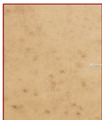
CuSn8 with Composition Sn 8 % P < 0.05 % Cu Rest
