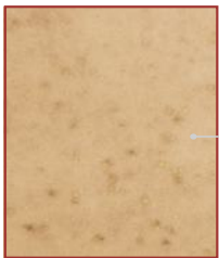
CuSn8 with Composition Sn 8 % P < 0.05 % Cu Rest
