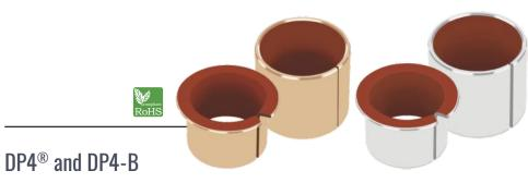
These self-lubricating metal-polymer bearings are particularly suitable to maintenance-free dry operation. They also offer exceptionally good performance in heavy-duty oil-lubricated applications. DP4-B bearings provide the added benefit of an antimagnetic, corrosion-resistant bronze backing. These lead-free products comply with EVL, WEEE and RoHS specifications.
