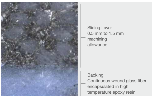
Fig. 3: HPMB® bearing microsection
