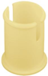
Plain bearings also may be made of [engineered plastics](#), which provide excellent wear resistance and low friction in both dry and lubricated operating conditions. Being injection molded, they can be designed to almost any shape and produced from a variety of resins compounded with reinforcing fibers and solid lubricant. These bearings exhibit excellent dimensional stability, low coefficients of friction and good thermal conductivity.
