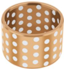
**Monometallic, bimetallic and sintered bronze plain bearings** are designed for use in both land-based and submerged industrial applications under high load with slow speed movements. **Solid bronze bearings** impregnated with lubricant provide maintenance-free performance in high temperature applications, whereas monometallic and bimetallic bearings are designed for lubricated applications.
