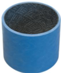
**Fiber reinforced composite bearings** are another form of plain bearing that consists of a filament-wound, fiberglass-impregnated, epoxy backing with a variety of low-friction, wear-resistant bearing linings. This structure enables the bearings to support high static and dynamic loads, while their inert nature makes them suitable for corrosive environments.
